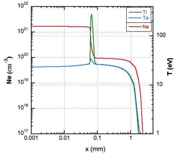
**Fig. 1.** 1-D MULTI simulation of a radiative shock in xenon at 20 ns, in the frame of a uniformly moving piston with a speed of 50 km/s. The initial conditions are a xenon density of  $\rho = 1.5 \times 10^{-3}$  gcm<sup>-3</sup> and a temperature of  $T = 300$  K.
