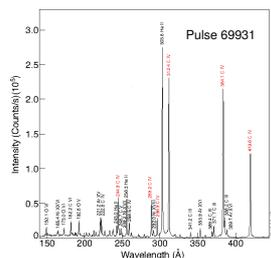
• Spectrum of JET pulse 69931 averaged between times 12.3 and 12.6 s showing the 6 VUV C IV spectral lines used, at wavelengths of 245 Å, 289 Å, 297 Å, 312 Å, 384 Å and 420 Å.
